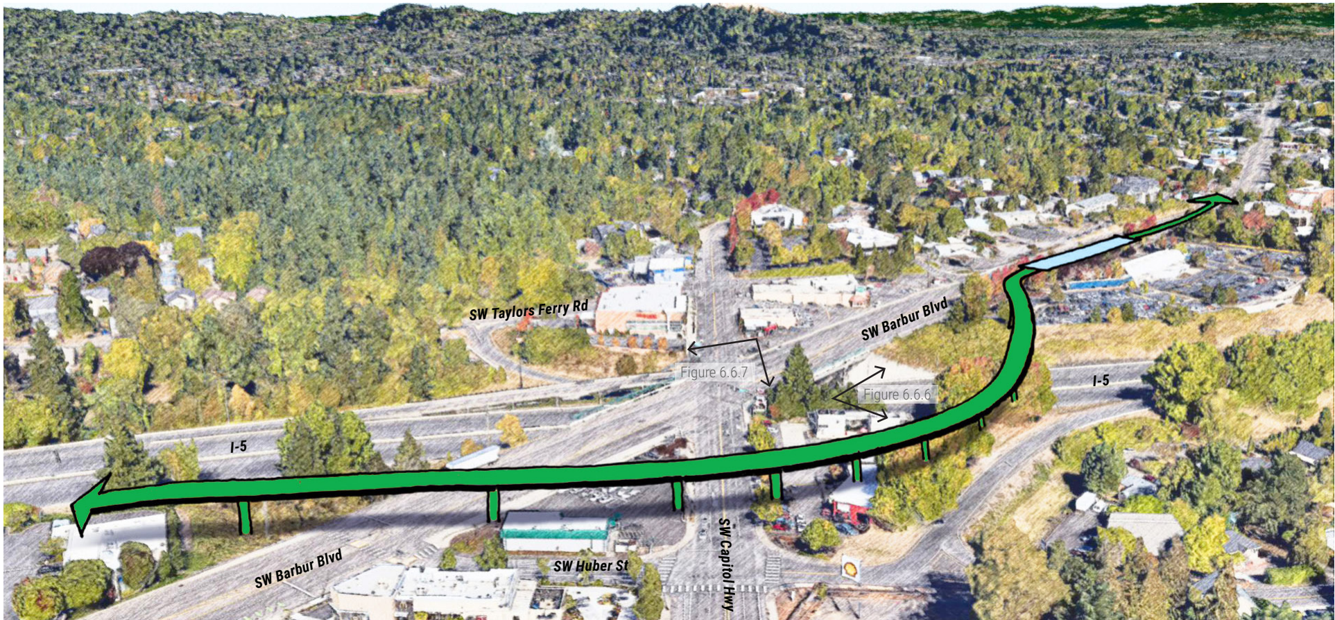
Figure 6.6.5 I-5 / SW Barbur Blvd Intersection Crossing
