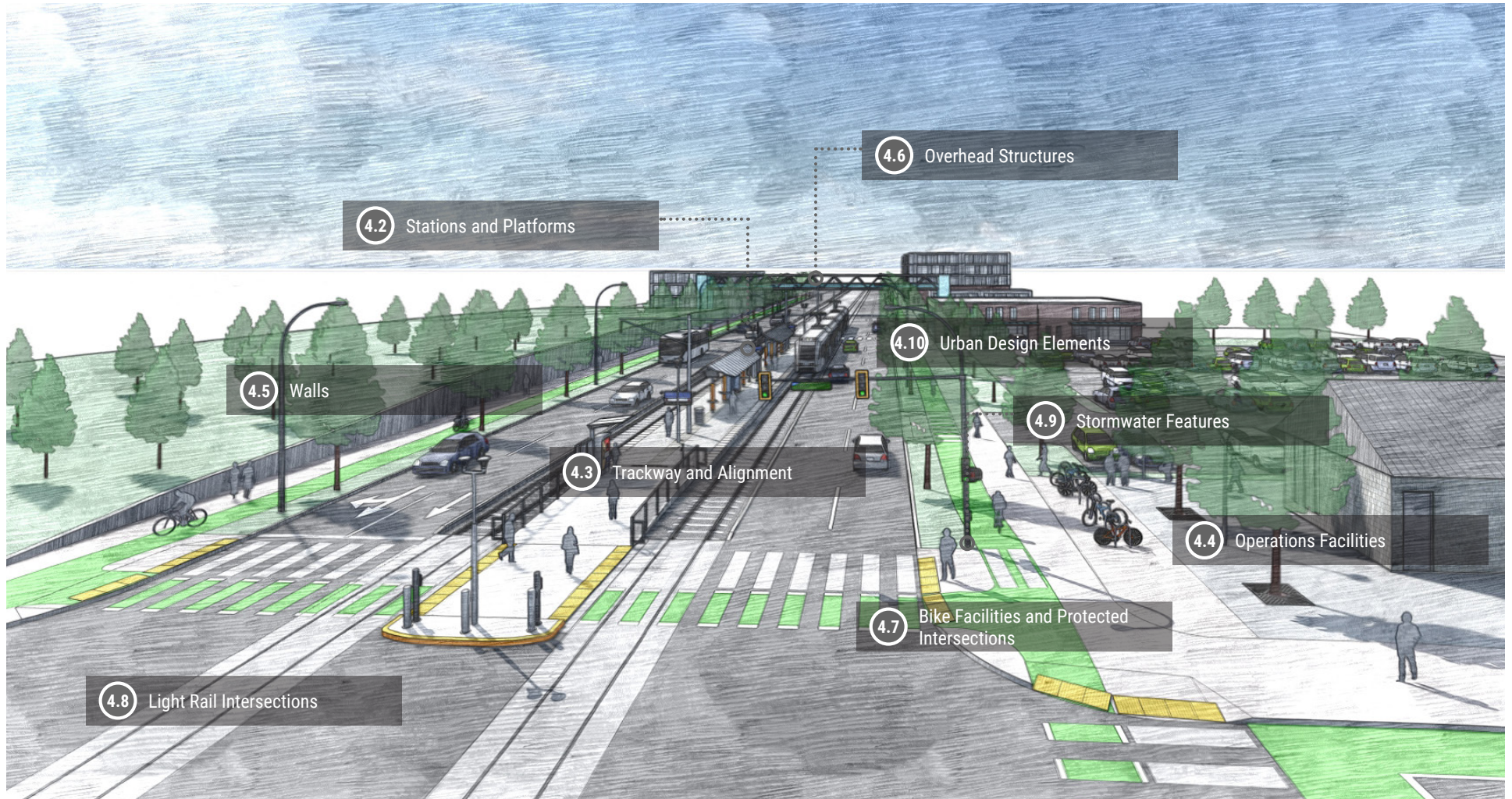
Figure 4.1: Typical Design Elements within a Station Area (this illustration is not representative of any location along the Southwest Corridor)
